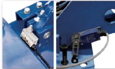
2 Upper & lower limit switches improve operator safety and lift longevity.
